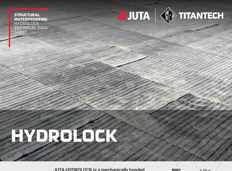
JUTA HYDROLOCK is a mechanically bonded Geosynthetic Clay Liner (GCL) composite of pulverised bentonite embedded between to layers of geotextile. The internal 5 kg of natural sodium bentonite swell sin contact with water to form a low permeability waterproofing barrier.
