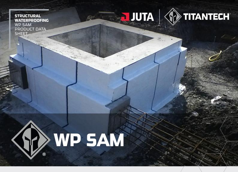
WP SAM, waterproofing self adhesive membrane, is a bituminous water proof sheet, which provides resistance to Radon, composed of self-adhesive SBS polymer modified bitumen with an upper surface finish of cross laminated HDPE and a lower surface finish of paper release film.
