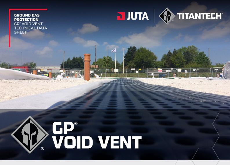
GP® VOID VENT is a cuspated HDPE core with a geotextile filter/separator bonded to a single side, in either 25 mm or 45 mm depth. The intended use of the void vent is to provide a means of ventilation when used in conjunction with an approved gas protection barrier, in accordance with the recommendation(s) contained within NHBC guidance and BS8485:2015 + A1 2019.
