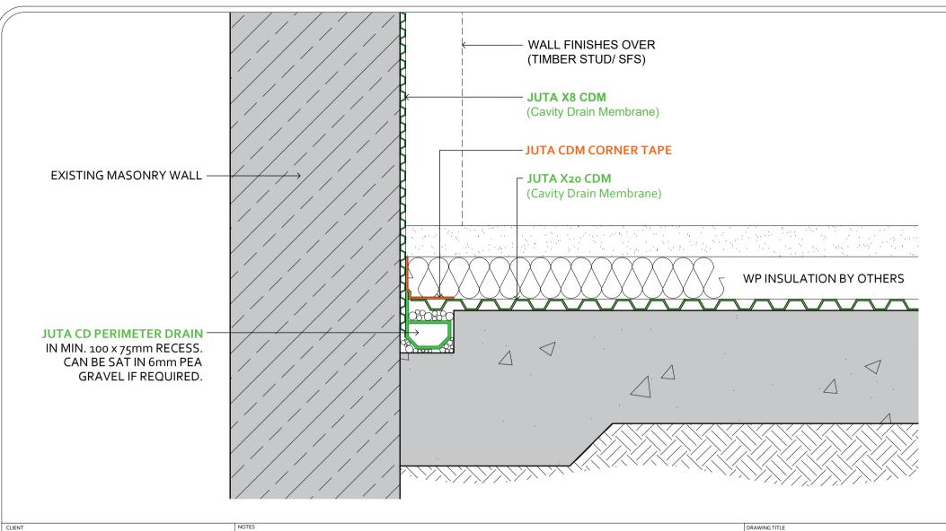
PROJECT Cavity Drain Standard Details
