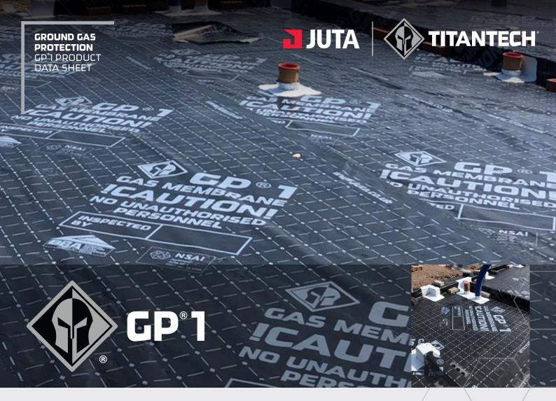
GP®1 proprietary gas resistant damp proof membrane (DPM) is a multi-layer, low density polyethylene membrane, reinforced with a polypropylene reinforcing grid with an integral aluminium foil for protection against methane, carbon dioxide, radon, ground gas, air & moisture.
