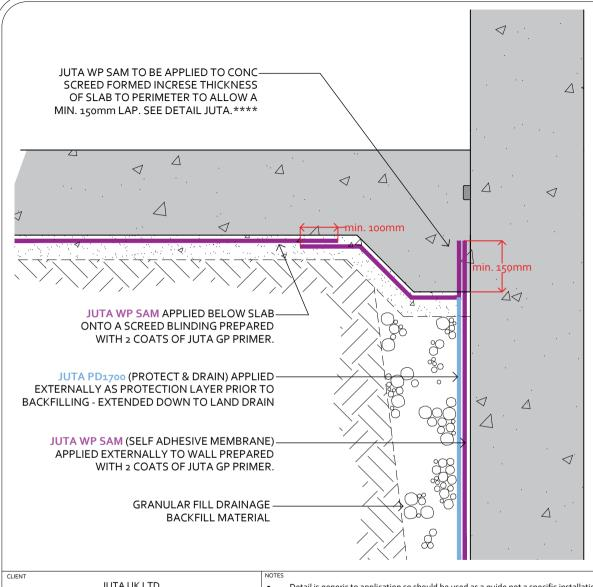
FOR VERTICAL TO HORIZONTAL LAPPING TRANSITIONS, THE SLAB SHOULD BE THICKENED BY 150mm WHERE LAPS BETWEEN MEMBRANES OCCUR WITH A CONCRETE SCREED BELOW TO APPLY MEMBRANE TO.
