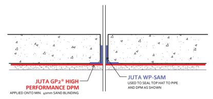
**ROD/ REBAR/ HANGAR WITH SELF ADHESIVE GAS MEMBRANE**
